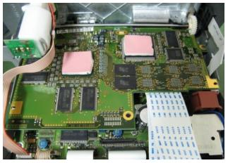
2. The connector which is pulled out the original FPC cable connect with second offered FFC cable. (The other side of second offered FFC cable connect with offered sub-board "LCD IN"
